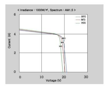
Current-Voltage characteristics of Photovoltaic Module SM-70KSM at various irradiance levels
